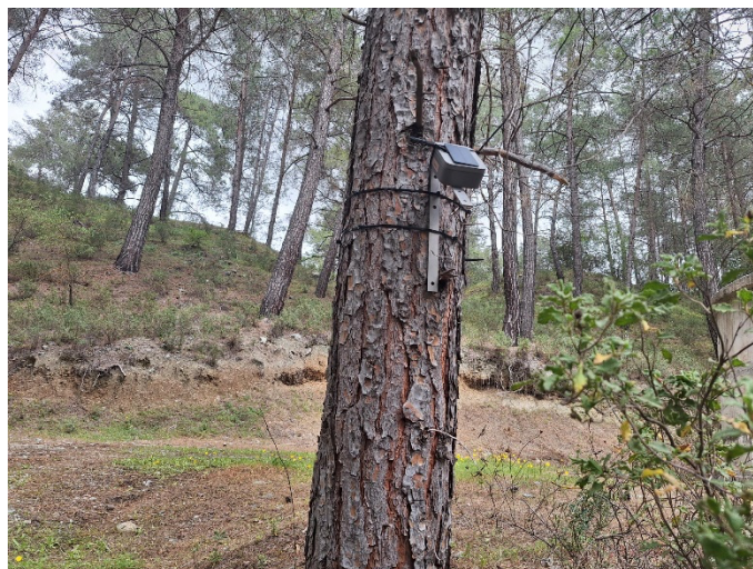
Figure 6: In-situ audio recognition module installed deeper inside the forested areas.
